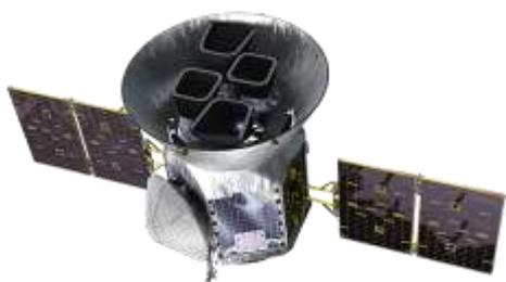
The TESS payload comprises 4 identical cameras of 10cm aperture with their fields of view consecutively aligned (covering 90 degrees of latitude). The spacecraft will be inserted into a highly eccentric and inclined orbit moving between the Earth and the Moon's orbit. While each orbit takes 13.5 days, the spacecraft will be able to spend 27 days looking at a single band of celestial longitude before moving to the next. In this way, an entire hemisphere can be mapped in a single year.
